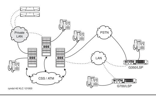
Because the G700 and G350 rely on IP Telephony technology, this option is especially attractive to customers who decide to use a majority of IP endpoints at the remote site. This solution will, however, continue to support analog endpoints and DCP endpoints. Analog trunks and ISDN trunks are also supported. To decrease operational expenses, the circuit-switched trunks back to the main site can be replaced with IP trunks.
